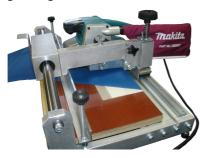
9. Please adjust the belt grinder in such a way that the front belting edge is slightly in contact.
