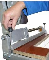
6. Please insert the prepared belt material in the grinding machine positioning the carrying side from the top to the backside and flush fit it on double-sided adhesive tape of the front cutting edge.
